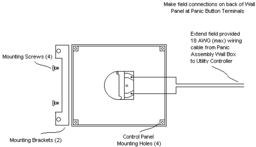
**Wiring the Panic Assembly Panel to the Wall Box:**
