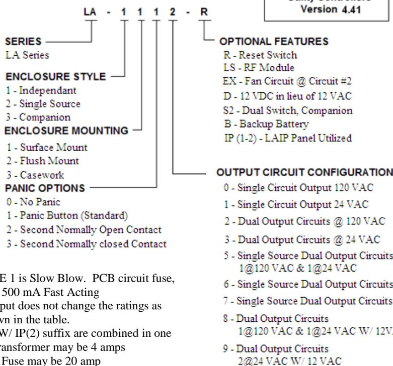
Output fuse on PCB, FUSE 1 is Slow Blow. PCB circuit fuse, FUSE 3 is 500 mA Fast Acting
