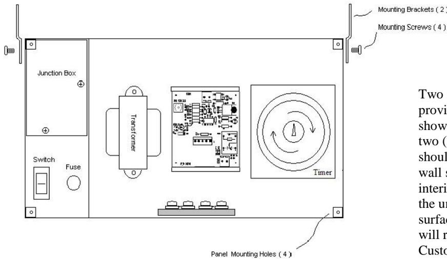
Two mounting flanges with screws are provided with the unit. Attach flanges as shown above. Then, fasten unit between two (2) wall studs. The face of the box should be even with the face of finished wall surface. After mounting unit, protect interior of box from construction debris. If the unit is to be surface mounted, separate surface flanges are required, and the unit will require drilling. Contact *ISIMET* Customer Service to obtain flanges.
