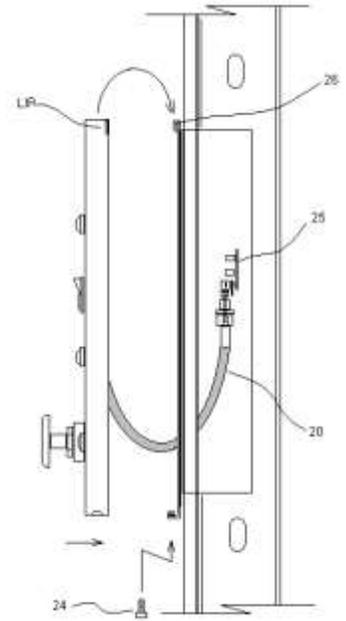
**Figure 16 – Wall Panel Installation Side view**
