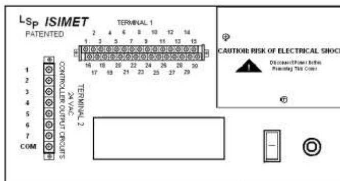
Note: All output circuits use a common "COM" terminal connection plus a specified connection post. See page 11 for switch to terminal post configuration
