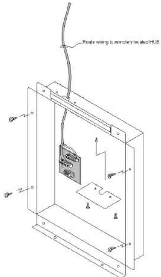
Figure 10 – Wall Box Wiring Installed
