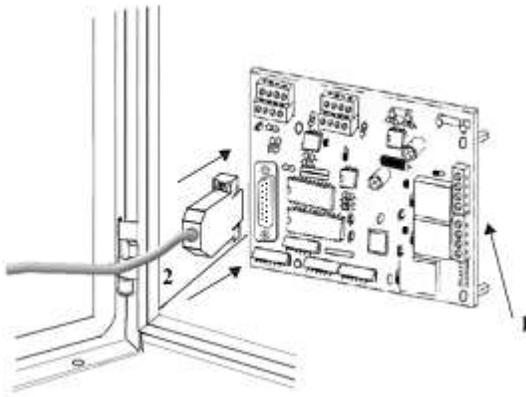
**The Version 9.1 PCB are configured so that this connector is positioned vertically along the inner side of the enclosure.**
