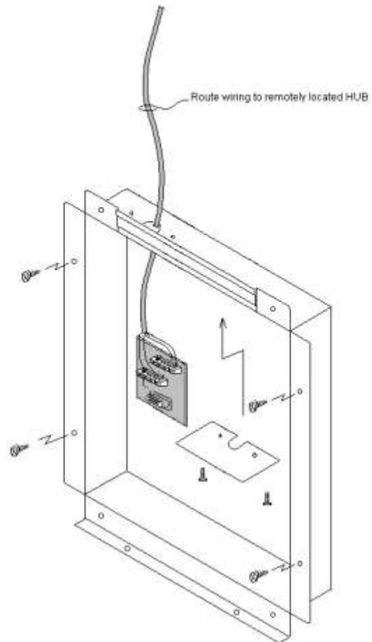
Figure 10 – Wall Box Wiring Installed
