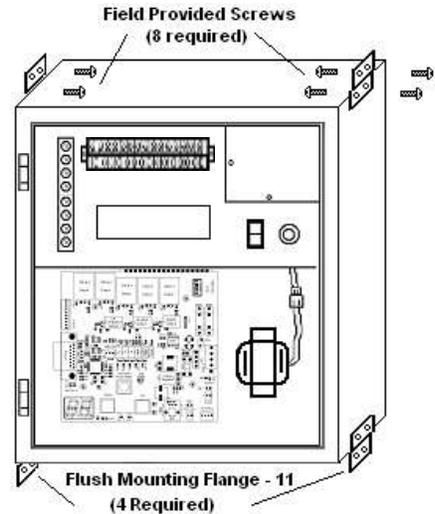
For best Flush Mounting results, recess face of enclosure's lip 1/4" behind wall finish
