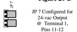
JP 7 Configured for 24-vac Output @ Terminal 1, Pins 11-12
