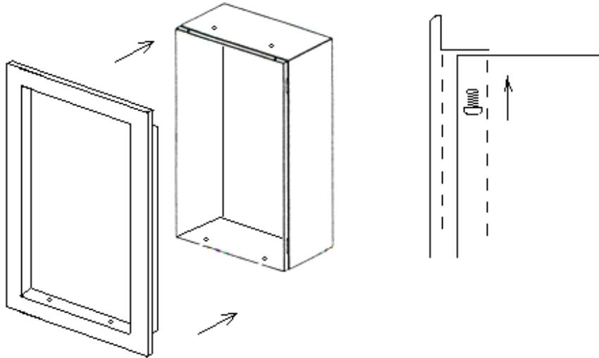
Prior to installing Door Trim, ensure that wall finishes are complete and that the door panel has been installed according to manufacturer's instructions. Verify that there is a 1/2" clearance from wall framing and sheet-rock or other wall surface material around the outer surface of the unit in order to permit the trim to be properly installed.
